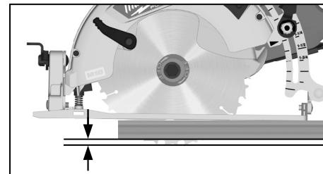
Adjust the cutting depth to the thickness of the workpiece. Less than a full tooth of the blade teeth should be visible below the workpiece.
