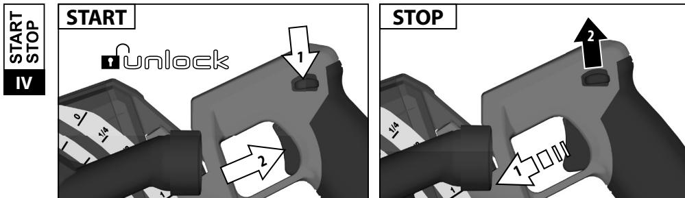
For safety reasons, the power tool is fitted with a switch lock and the on/off switch cannot be locked in the ON position.
