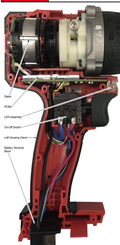
Be sure that all mechanical and electrical components are placed firmly and squarely in corresponding cavities of left housing halve.
