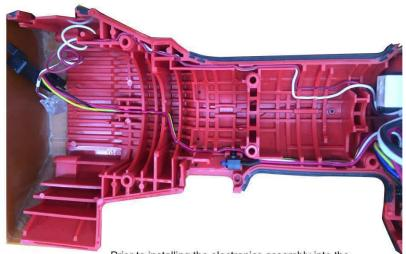
Prior to installing the electronics assembly into the housing support, place grounding terminal over screw boss as shown. Route ground wire, removing as much slack as possible. Be sure wire is pressed firmly to the back of the wire traps.
