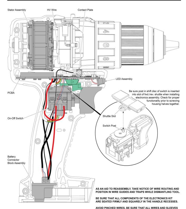
ARE PRESSED COMPLETELY DOWN IN WIRE GUIDES AND TRAPS.
