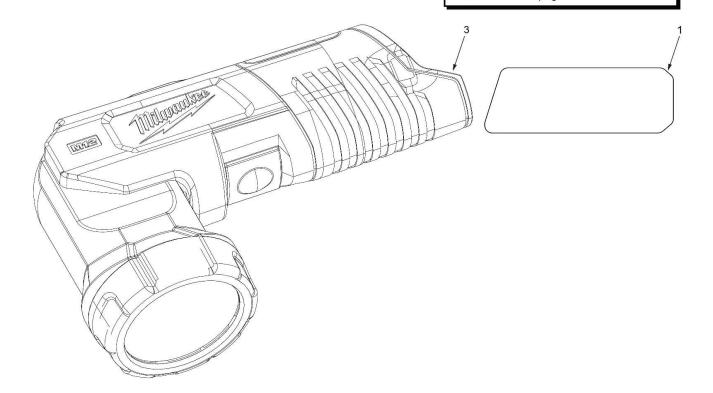
A clean, dry surface is essential for proper performance for any adhesive system. The area intended for application of any adhesive label or nameplate must be prepared by cleaning with isopropyl alcohol. The solvent is to be applied with a clean, lint free applicator and the surface allowed to dry before applying the label or nameplate.
